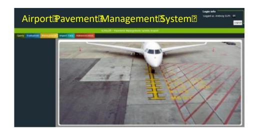
Web-based system, developed over a geographical information system (GIS), in order to allow remote access to all information for the pavement maintenance groups in the different positions/assets of administration and to allow the representation and use of all kind od data.
